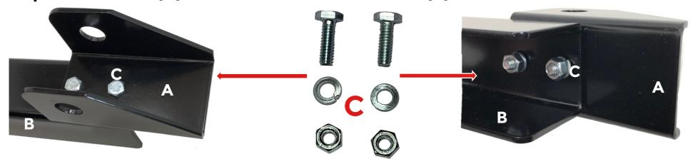
TOP VIEW: Use the 2) 1/4" x 3/4" bolts and insert them thru both holes with the receiver mount base
