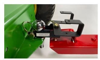
To haul hitch pin lawn and garden tools use the 3/8" center hole to secure equipment for towing. (3/8" - Hitch pin is not supplied)
